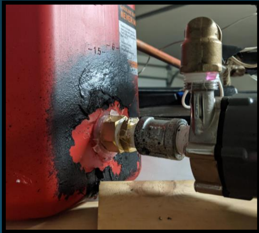
Figures 6a and b: Improved reservoir seal
