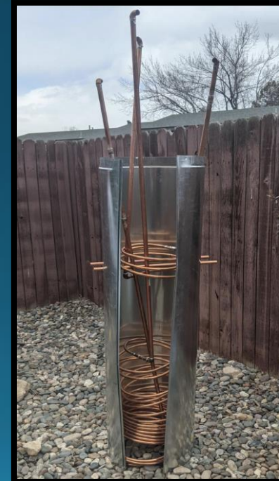
Figure 21: Finished HX Stack
