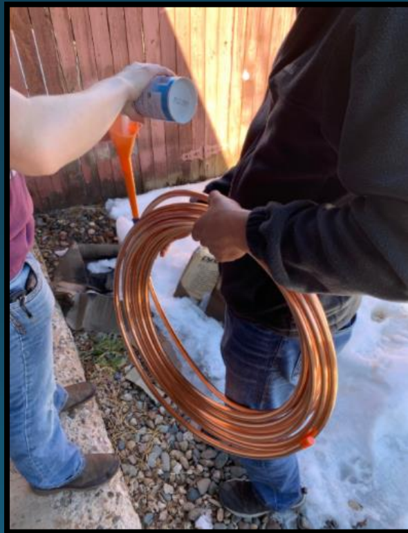
Figure 17: Salt in HX Coil
