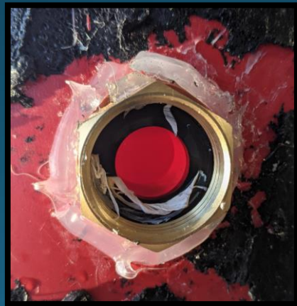
Figures 6a and b: Improved reservoir seal
